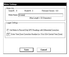
If the box below the logger name field is checked, the logger will store GPS data only if it has been differentially corrected. If the differential correction is not found, only the SPAD reading will be stored in the data file.
