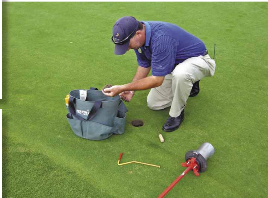
A cup cutter is used to create the hole for the Toro Turf Guard wireless sensor. Once the sensor is properly placed in the hole, it is filled in with soil and then the topped off with the turf plug.
