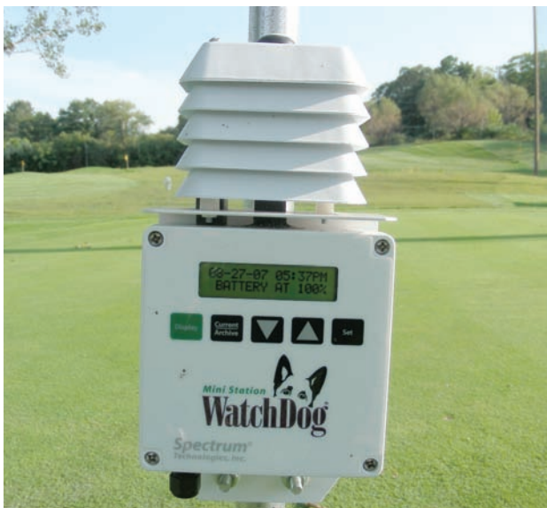
Figure 2. Close-up of the mini weather station with a light sensor used in this study.
