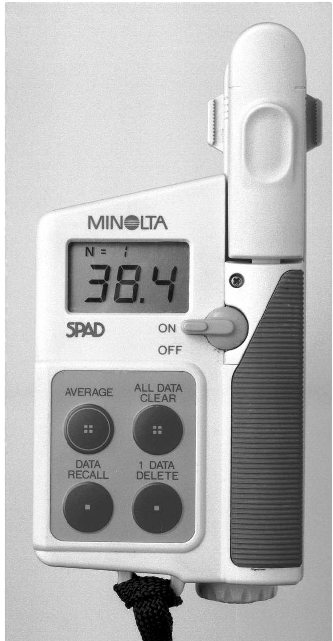
Figure 3. Picture of chlorophyll meter showing function buttons, display screen, and meter head.
