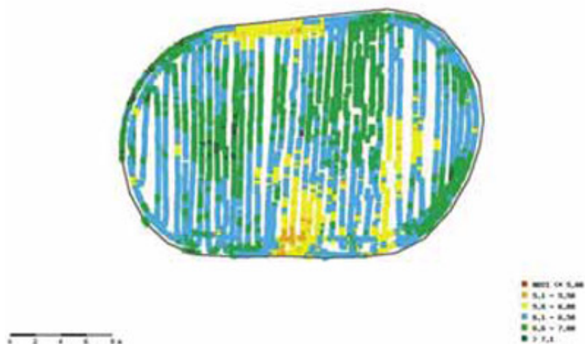
Image 1: Turfgrass health on a golf green measured with a reflectance sensor. Higher numbers equate to better plant health. Image courtesy of Dr. Dana Sullivan.
