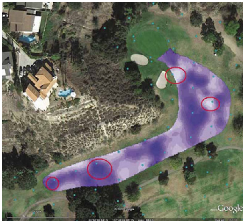
Image 4: A soil moisture map of a fairway with problem irrigation heads circled.
