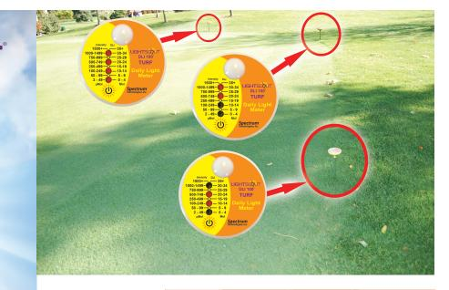
Use multiple DLI 100s to simultaneously compare light levels and the effect on turf health and quality.
