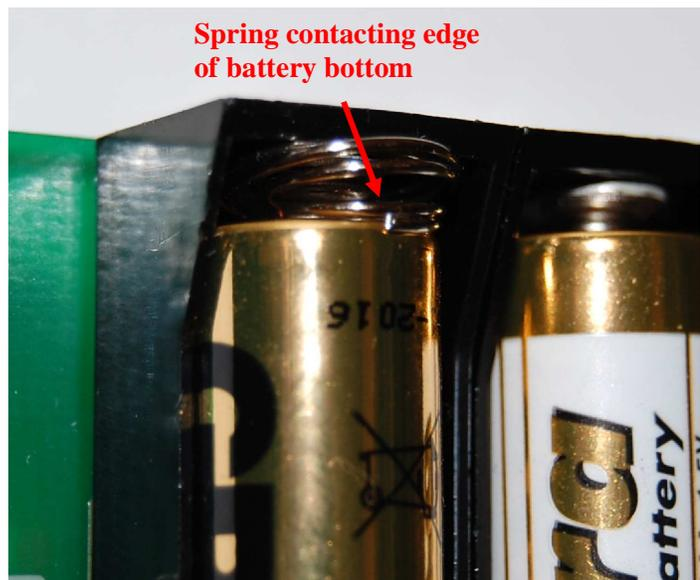
Figure 3. Example of a short circuit caused by the battery holder spring contacting the negative terminal of the battery (by design) and the positive terminal (by puncturing the plastic insulator).
