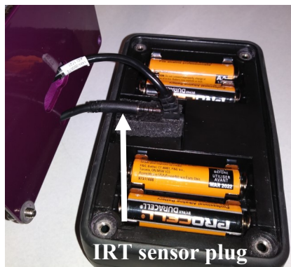
Fig. 2: IRT sensor inserted through flange
