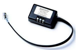
The Alarm Output Module (AOM) is a dry contact, control relay that operates as either a normally-open or normally-closed single pole switch. The output is rated at 1 amp AC or DC. It should be used with low voltage control signals due to its exposed terminal contacts.
