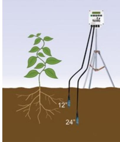
installed in the root zone. A single sensor should be placed in the middle of the root zone. When two sensors are installed at a single site, it is recommended to place one sensor at the top of the root zone and a second at the bottom. An advantage of installing multiple sensors is it allows you to see how well irrigation and rainwater is moving through the soil profile.
