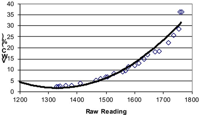
A calibration curve can also be obtained by gradually wetting a pre-measured amount of soil with known increments of water. Care must be taken to return the soil to its original bulk density before a sensor reading is made.
