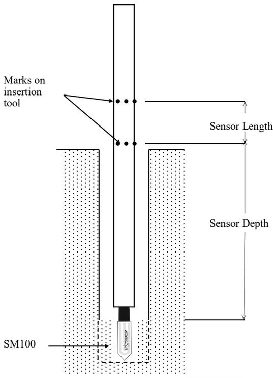
The access hole should then be carefully backfilled with native soil and tamped down to eliminate air pockets.
