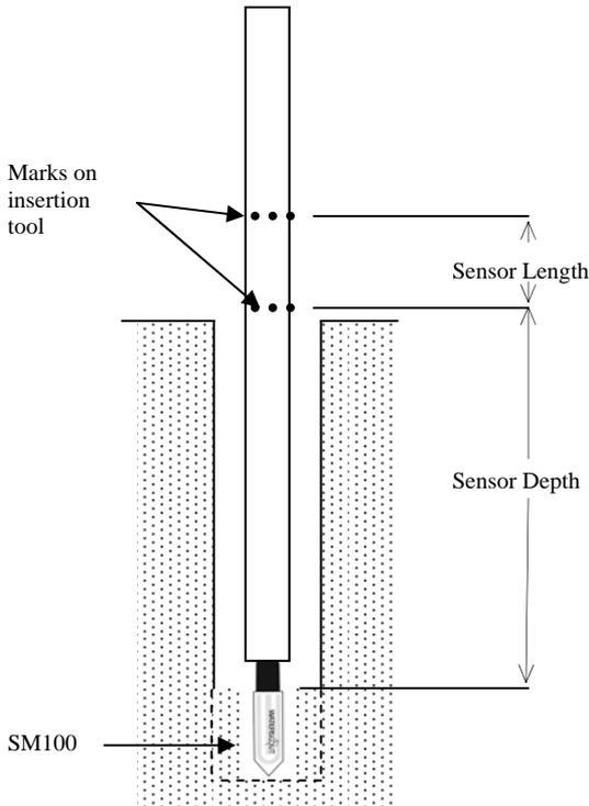
The access hole should then be carefully backfilled with native soil and tamped down to eliminate air pockets.
