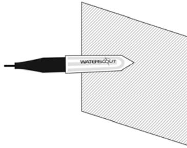
be taken to avoid snapping it during installation. To limit the effect of water moving vertically through the soil profile, the sensors should be installed so the flat face is perpendicular to the soil surface. For the same reason, if sensors are installed at multiple depths, they should be offset from one another.
