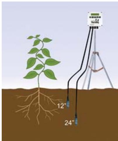
or two sensors should be installed in the root zone. A single sensor should be placed in the middle of the root zone. When two sensors are installed at a single site, it is recommended to place one sensor at the top of the root zone and a second at the bottom. An advantage of installing multiple sensors is it allows you to see how well irrigation and rainwater is moving through the soil profile.
