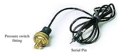
The Irrigation On/Off sensor is designed to work in conjunction with the WatchDog dataloggers and Weather Stations. The pressure switch trips **ON** at 5 PSI (+/- 1.0 PSI). Because the sensor must be plumbed into the irrigation line, your station should be located at a place in the line where this can be done conveniently and cleanly.
