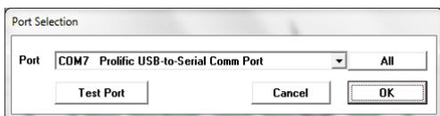
The computer **Communications Port** to which the PC-3.5mm serial cable is connected
