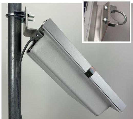
The solar panel bracket attaches to a post or pipe using the U-bolt (fig. 2). The U-bolt can accommodate a post diameter of 1.37 inches (3.5 cm) or less.
