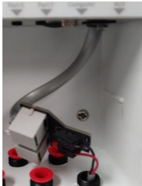
Figure 6: Adapter attached to AUX port
