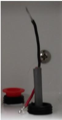
Figure 5: Power cable through gland
