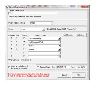
The logger continues recording data even when the **WatchDog Properties** screen is opened. If the **OK** button is clicked, any configurations are saved, the data is cleared, and data collection restarts. If the **Cancel** button is clicked, the logger configuration is not updated, no data is cleared, and the logger continues logging.
