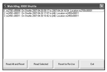
tions. Each line contains the model number, serial number, the time it was offloaded to the Data Shuttle, the oldest datapoint offloaded (or "(All)" if everything was offloaded), and the location name.
