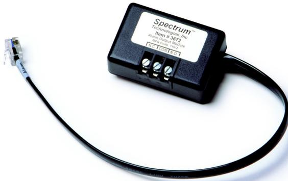
The Alarm Output Module (AOM) is a dry contact, control relay that operates as either a normally-open or normally-closed single pole switch. The output is rated at 1 amp AC or DC. It should be used with low voltage control signals due to its exposed terminal contacts.
