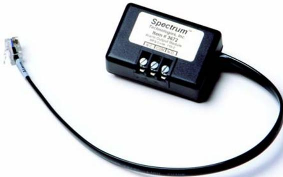
The Alarm Output Module is a dry contact control relay that operates as either a normally-open or normally-closed single pole switch. The output is rated at 1 amp AC or DC. It should be used with low voltage control signals due to its exposed terminal contacts.
