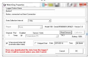
Set the data collection interval ranging from 1 to 120 minutes and ensure all channels are enabled. The Delay Start option allows you to start logging data at a later time.
