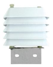
Thank you for purchasing a Digital Temperature/RH Sensor. The sensor was designed to be compatible with the WatchDog Sensor Pups (Item 3900, 3960, and 3930) or the pre-packaged Sensor Pup Stations. To ensure the sensor outputs accurate meteorological data, the sensor is housed inside a radiation shield.
