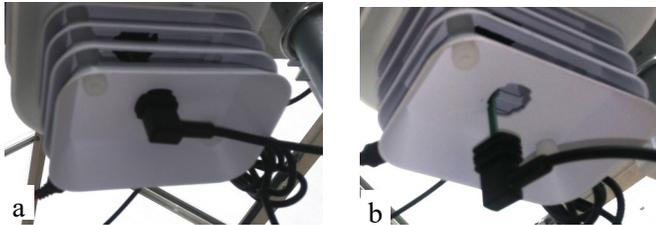
Fig. 4: T/RH sensor a.) installed and b.) uninstalled
