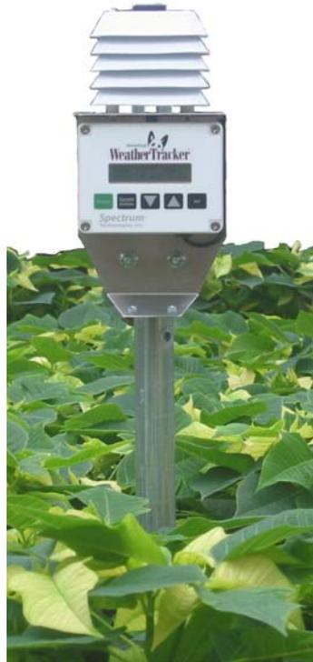
*Figure 1: WeatherTracker mounted on 1" conduit*
