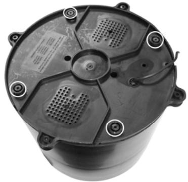
Set the bracket on the collector, lines up the holes in the bracket with those in the collector. If only two of the four holes line up, rotate the bracket 1/4 turn. Attach the bracket to the collector using the four machine screws included.
