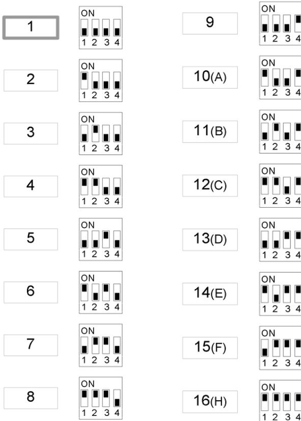
*Dip switch configuration for sensor ID*
