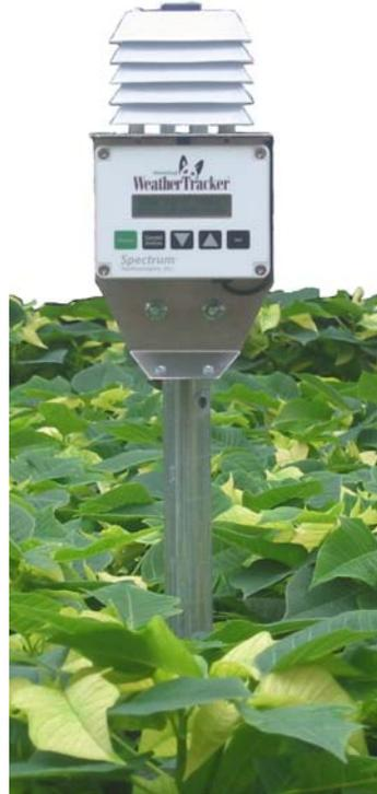
Figure 1: WeatherTracker mounted on 1" conduit
