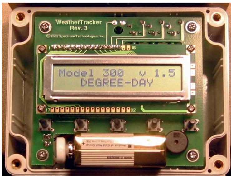
Figure 2: WeatherTracker Battery Compartment
