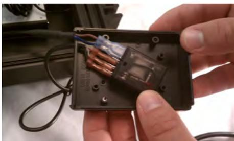
Plug the sensor cord into the sensor port. Adjust the relay/housing to fit in the case. Tighten the gland nut. Close the case.
