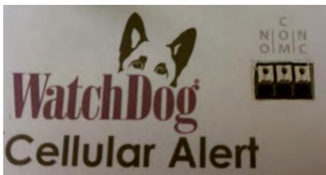
To insert the wires, press on the white button and insert the wire into the corresponding terminal. Release the button when the wire is in place to lock it. **To avoid short circuiting, ensure that no bare wire is exposed above the terminal block.**
