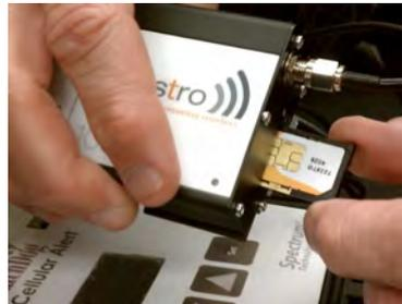
The CDMA modem does not require nor have a SIM card holder. When activating the unit your service provider will need the modem's ESN and MEID number listed on the back. The CDMA modem has two identical connectors on top. Use the one labeled 'CDMA' for the antenna.
