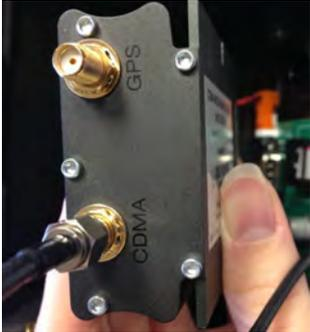
Slide the module into the DB15 connector and then snap it onto the Velcro at the back of the case. Reattach the antenna to the Velcro at the top of the case.
