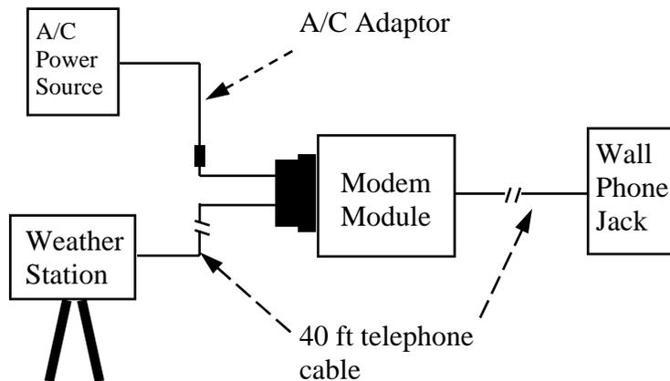
Figure 1. Connection diagram for the dial-up modem
