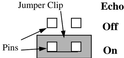
Figure 2: Top view of Echo On/Off switch
