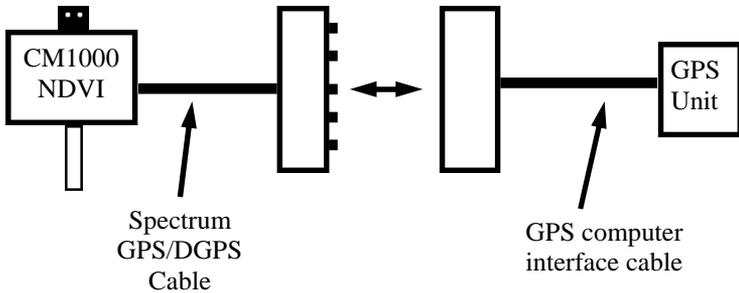
Connecting the CM1000 NDVI meter to a GPS unit
