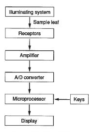
Figure 2: Block diagram of the SPAD-502Plus
