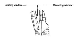
Figure 4: Illuminating/measuring system of the SPAD-502Plus
