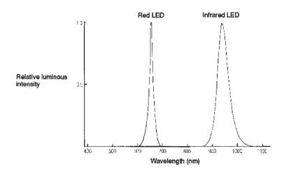
Figure 3: LED luminous intensity characteristics
