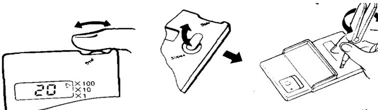
apply the standard 15 X 10 SLOPE solution as in step (3). After the readout has stabilized, pull the rubber plug and use the driver end of the tweezers to adjust the SLOPE until the display reads 15 X 10.
