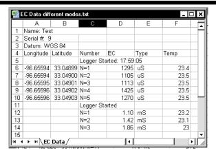
Sample data showing results of data collected with and without GPS activated. Note: GPS signal not found when recording data in lines 12 through 14.
