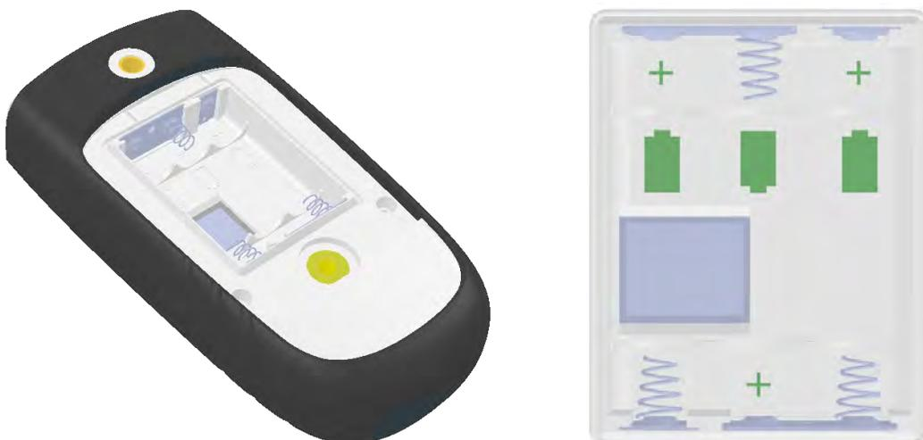
It is possible to temporarily install non-rechargeable batteries when the rechargeable batteries have run out and there are no other fully charged rechargeable batteries available (i.e. when using the meter in a remote location). This should be done with care as the non-rechargeable batteries should be removed immediately after use and before the meter is connected to a power adaptor or USB port.
