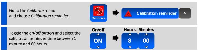
Confirm and apply with the *Set* button, or exit with the *Back* button to discard any changes.
