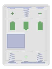
It is possible to temporarily install non-rechargeable batteries when the rechargeable batteries have run out and there are no other fully charged rechargeable batteries available (i.e. when using the meter in a remote location). This should be done with care as the non-rechargeable batteries should be removed immediately after use and before the meter is connected to a power adaptor or USB port.
