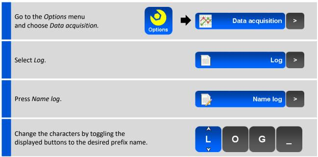
Confirm and apply with the *Set* button, or exit with the *Back* button to discard any changes.
