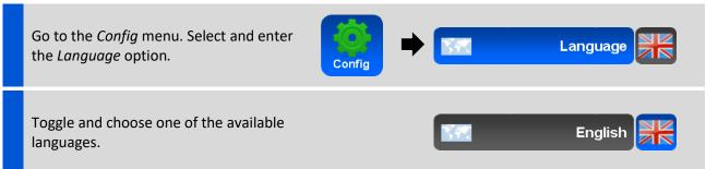
Confirm and apply with the *Enter* key, or exit with the *Back* key to discard any changes.
