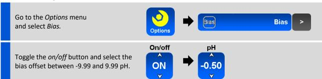
Confirm and apply with the *Set* button, or exit with the *Back* button to discard any changes.
