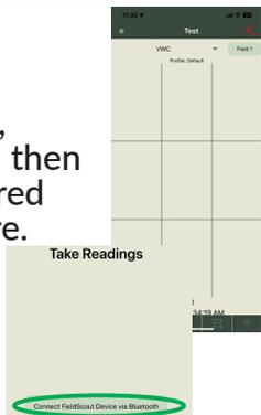
Initiate pairing by tapping **Connect FieldScout Device via Bluetooth**.
