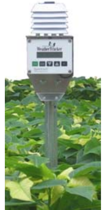
Figure 1: Weather Tracker mounted on 1" conduit
