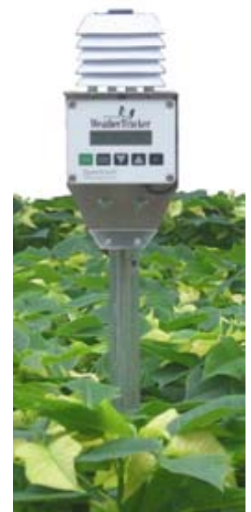
Figure 1: WeatherTracker mounted on 1" conduit
