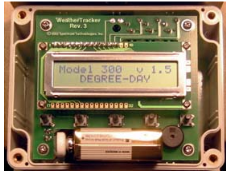
Figure 2: WeatherTracker Battery Compartment
