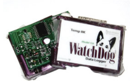
WatchDog Model 110 Data Logger accidentally crushed by a vehicle. Saved data was successfully retrieved!
