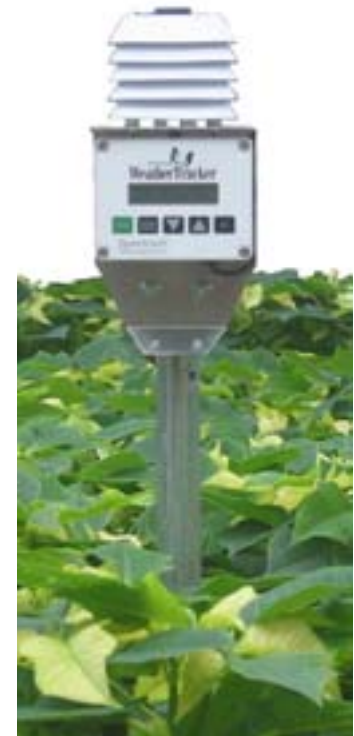
Figure 1: WeatherTracker mounted on 1" conduit
