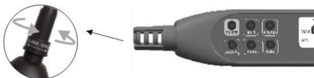
**Note:** Be sure to rotate the sensor cap to open it.
