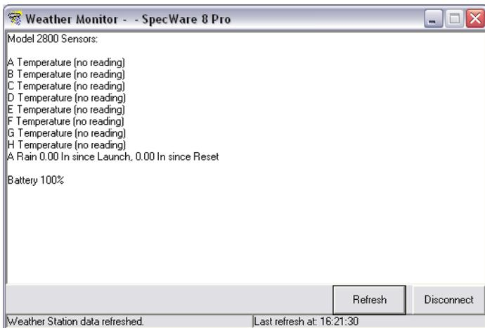
Monitor screen generated by toolbar quick-button for a Model 800 station.
