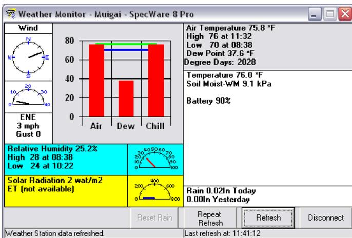
Monitor Screen generated by WatchDog Manager screen. Note: This is the only option available for the 1000 or 2000-series mini- and the weather station.
