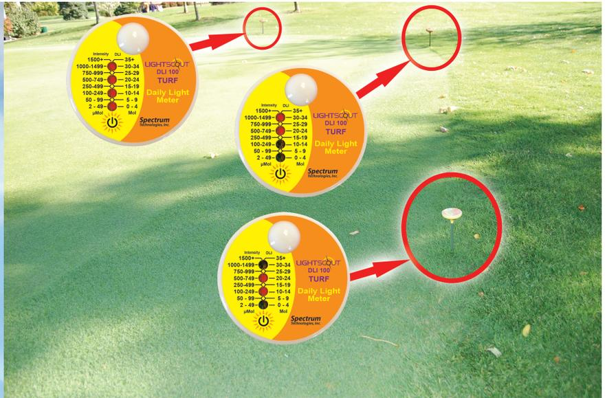
**Use multiple DLI 100s to simultaneously compare light levels and the effect on turf health and quality.**
