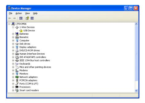
If the driver is not installed correctly then the device will show up as a yellow exclamation point.
